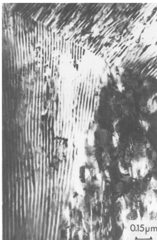
Figure 6 Parallel alternate lamellae of  $\theta$  and aluminium-copper solid solution, from ion-beam thinned specimen of Al-17.3 at. % Cu.
